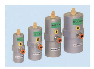
A spring is incorporated in the body to ensure self starting when used in conjunction with a self exhausting valve. The vibrator requires a minimum of 30 PSI to operate.
