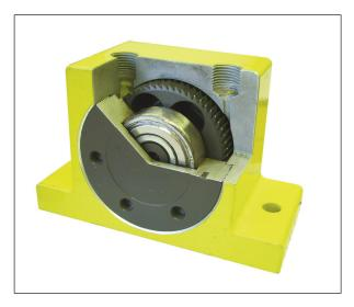
Vibration is produced by the centrifugal force of the positive and negative unbalanced moments in the rotor. The rotor is supported on two heavy duty pre-lubricated matched sealed bearings. A special high performance grease ensures a long working life.
