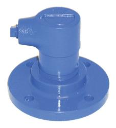
Ensure air supply is filtered and lubricated. Use ¼" bore hose. If it is not connected to an automatic filter / lubrication, pour 5ml of recommended oil (Tellus R10 or equivalent) into the inlet port every 8 hours.
