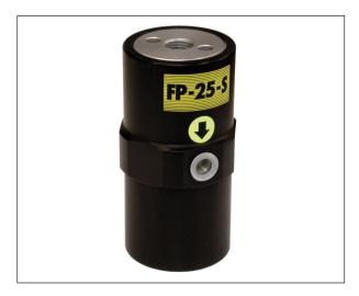
A spring is incorporated in the body to ensure self starting when used in conjunction with a self exhausting valve. The vibrator requires a minimum of 30 PSI to operate.
